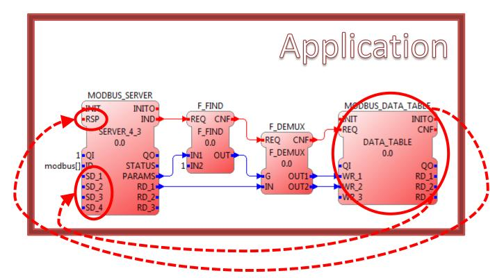
Not to mention that another complex Function Block network would connect the MODBUS\_DATA\_TABLE back to the MODBUS\_SERVER to take care of the MODBUS\_SERVER responses.
