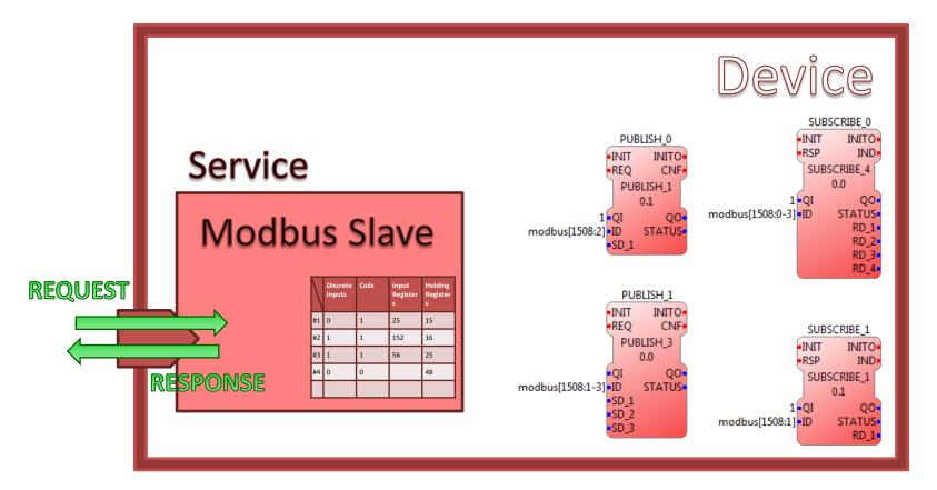
On the other hand the Modbus Slave Service will serve requests from the Modbus Master independently of the IEC 61499 Application.
