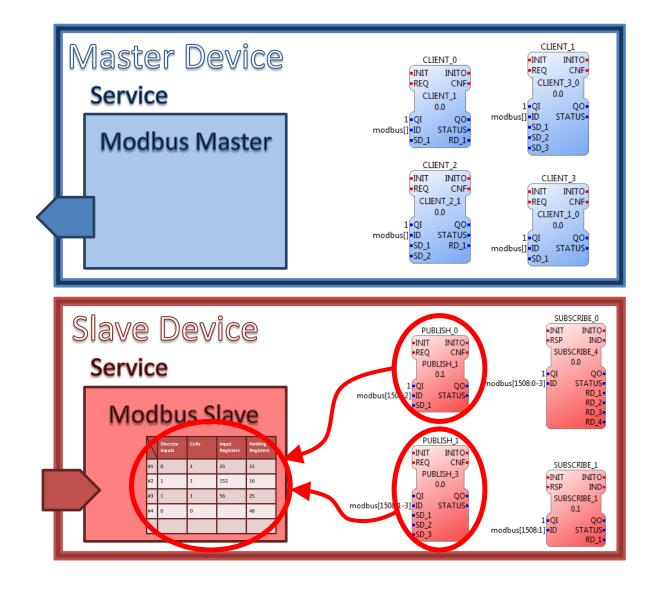
The application of the Modbus protocol with IEC 61499 Function Blocks in the proposed way:
