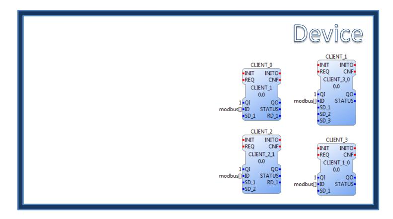
Instead multiple CLIENT FBs interacting with a single Modbus Master Service can be used.
