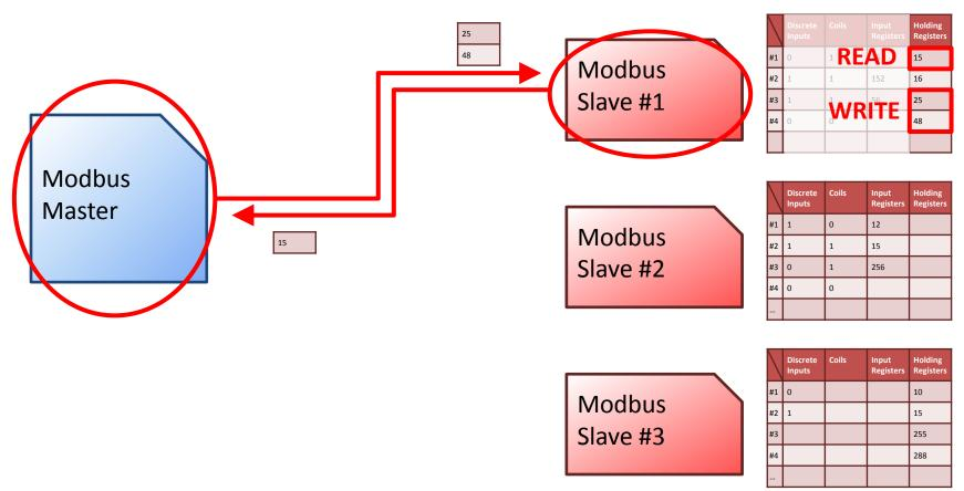
However the Modbus Master can only send a Read/Write request for Holding Register data.
