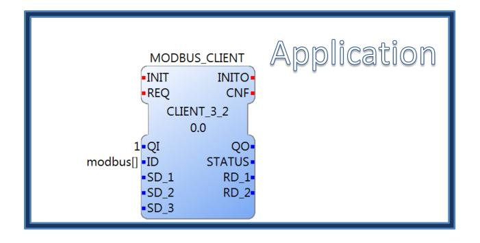
But implementing the Modbus Master with a single CLIENT FB comes to the same deadlock as the implementation of the Modbus Slave with a single SERVER FB.
