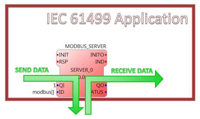
But having a single SERVER FB means that all Modbus input and output of the device is done by that single SERVER FB.
