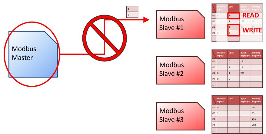
However the Modbus Master can only send a Read/Write request for Holding Register data.
