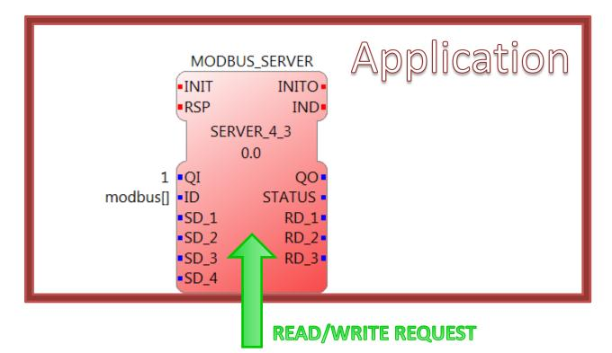
But then we would expect that device to receive only mixed Read/Write requests. This limits the Modbus data type to Holding Registers.
