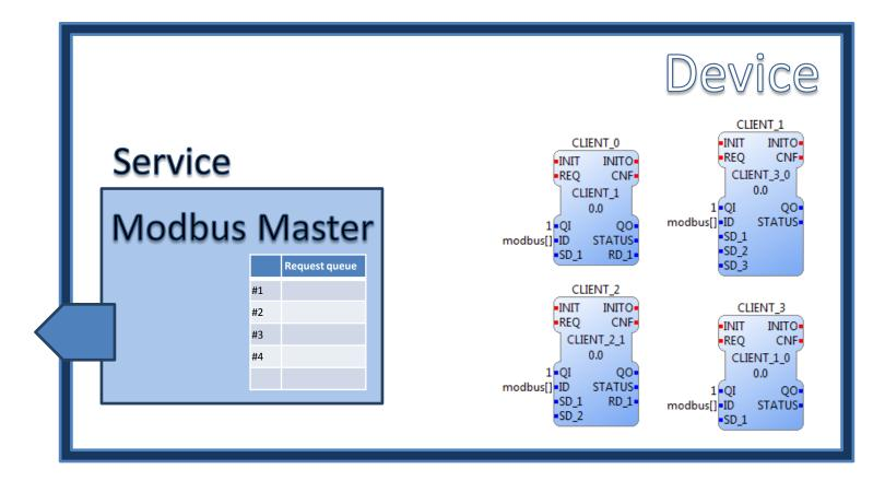
The Service will open a port for sending Modbus requests and create a queue to store requests registered by CLIENT Function Blocks.
