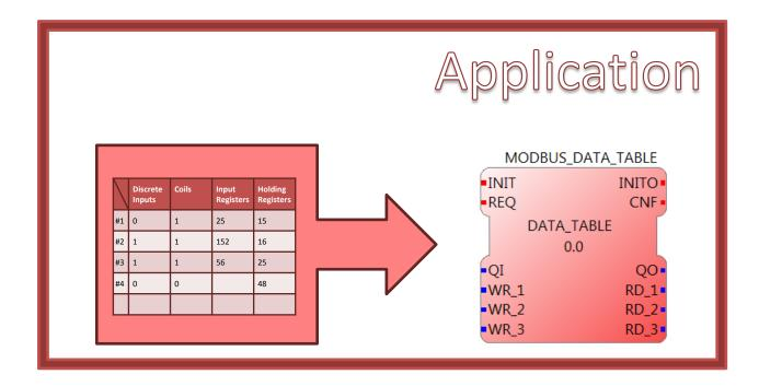
Moreover in such implementation the Modbus data table would be implemented inside the IEC 61499 Application's Function Block network as a special Function Block.
