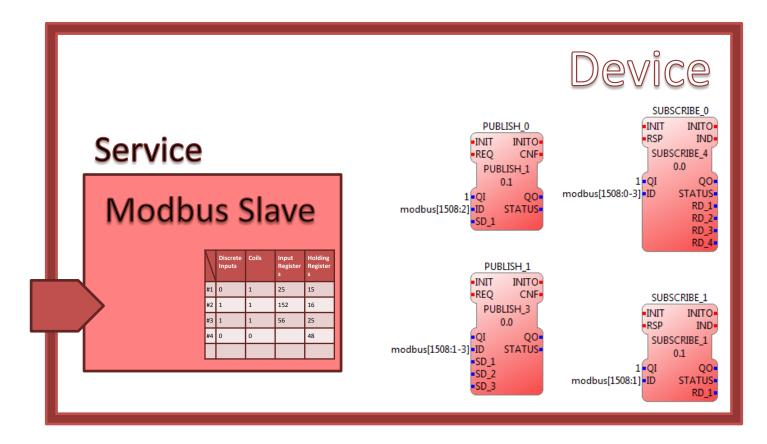
The Service will set a listening port for incoming Modbus requests and allocate some memory for the Modbus data table.
