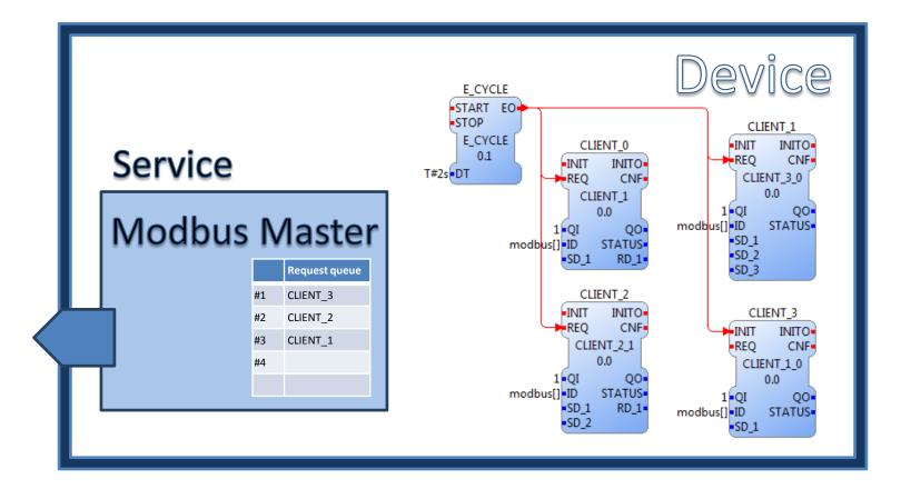
The IEC 61499 Application must take care to avoid long delays or the endless increase of the queue by using either a freewheel cascading scheme or the most common cyclic polling scheme.
