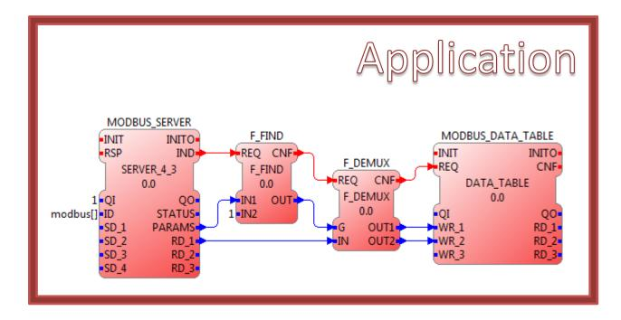
And finally the Application would interpret the parameters and connect the MODBUS\_SERVER with the MODBUS\_DATA\_TABLE using a complex Function Block network.
