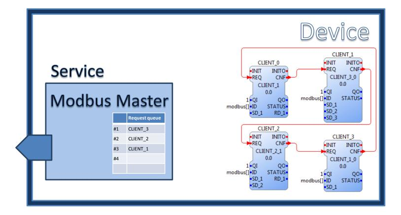
The IEC 61499 Application must take care to avoid long delays or the endless increase of the queue by using either a freewheel cascading scheme ...
