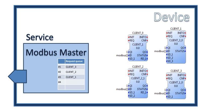
The top of the Request queue is picked. The request is sent. A response is received. The corresponding CLIENT FB is informed. The request is removed from the queue.
