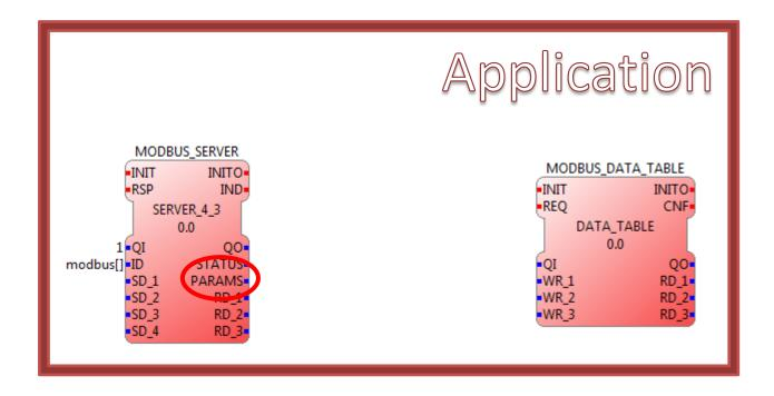
Modbus messages would enter the Function Block network as parameters in some string format.
