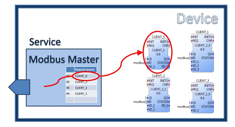
The top of the Request queue is picked. The request is sent. A response is received. The corresponding CLIENT FB is informed.
