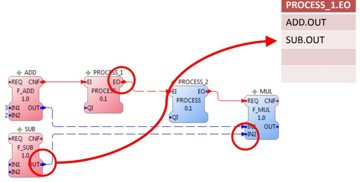
The event list corresponds to a point of device interconnection in the Function Block network.
