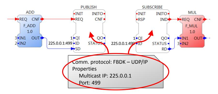
The development environment should offer an option to add and set the Communication Function Blocks automatically utilizing the programmers options.
