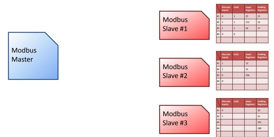
In each Modbus network only one Master can exist, but several Slaves can be connected.
