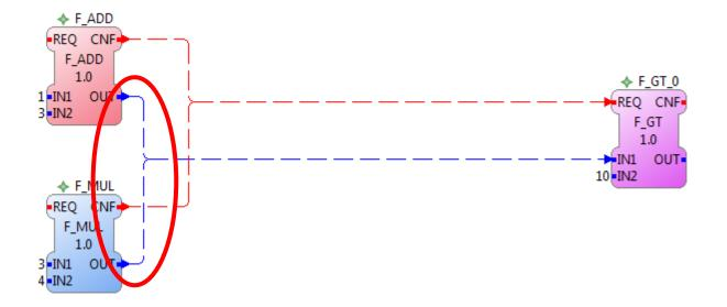
However to allow such configuration to result automatically the original design wouldn't be a legitimate IEC 61499 configuration.
