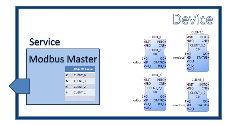
The Modbus Master can send only one request at a time so it picks the top of the Request queue and serves it.
