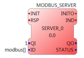
Trying to implement a Modbus Slave in IEC 61499 comes to the obvious solution of a single SERVER Function Block.
