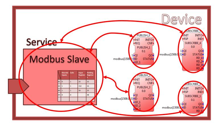
Many PUBLISH and SUBSCRIBE Function Blocks can be associated to a single Modbus Slave Service and function simultaneously.
