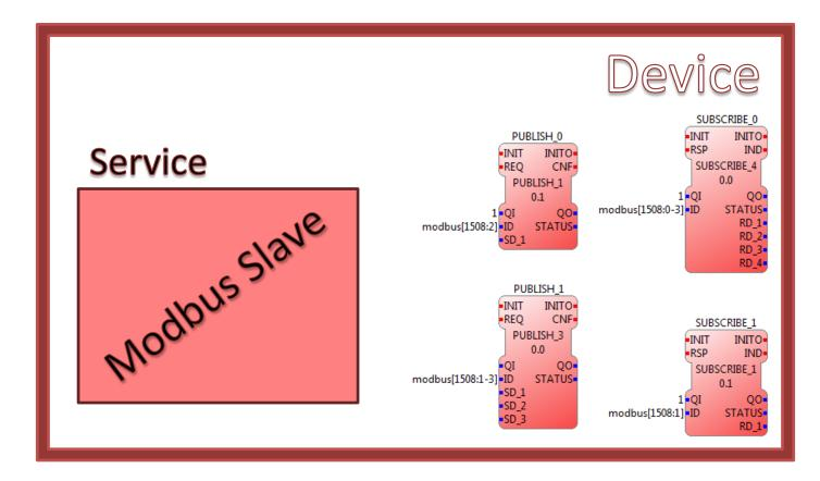
In such case the Modbus Slave is implemented as a Service inside the Device.
