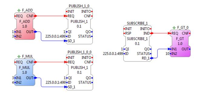
This configuration is legitimate according to IEC 61499 standard and allows a single SUBSCRIBE FB to receive data from two different PUBLISH FBs.
