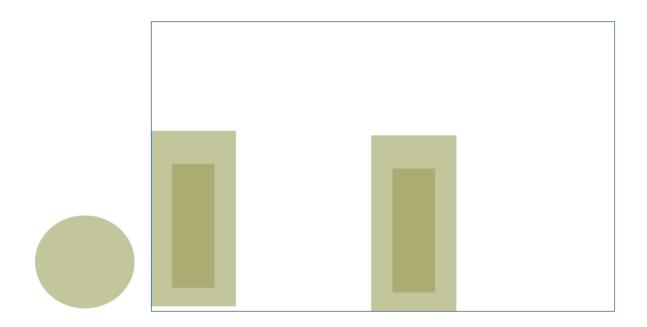
in an editor. The black rectangle represents the displayed area when the visualization is running. It has two light-green rectangles in it, representing the first and second buffer. The darker green rectangles inside will vary in height to show the number of items in each buffer.
