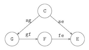
F is the factory being studied, generator G sends products into the factory, and exit process E retrieves finished products. The factory is tightly controlled by controller C that sends a signal to G or E before a product may be moved. The model is as follows:
