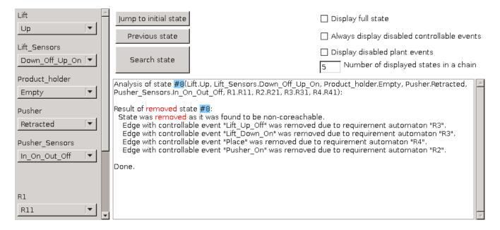
As expected, the analysis tools displays that the state was removed, apparently because it was not co-reachable. Again you get the list of removed edges from this state, as an aid to decide which requirement should be checked, if this was not expected.
