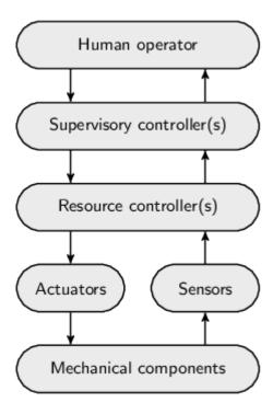
At the bottom are the mechanical components, such as motors, switches, levers and valves. Their operation can be steered through actuators and their state of operation can be observed through sensors. Resource controllers provide a first level of control. They may for instance correct for sensor jitter, translate continuous signals to discrete ones, or detect and even correct anomalous situations.
