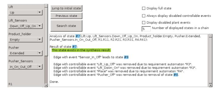
State #7 has one outgoing edge, leading to state #9 using event Sensor\_In\_Off. The last line with the removed controllable events displays a removed edge because destination state #8 was removed.
