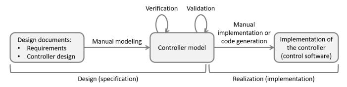
At the center is a controller model, a model of a controller that unambiguously specifies how the controller works. It precisely specifies how the state of the controller changes when a sensor signal changes, and under what conditions and in which states an actuator may be turned on or off. Ideally, the model has a mathematical foundation. It may for instance be modeled as one or more state machines.
