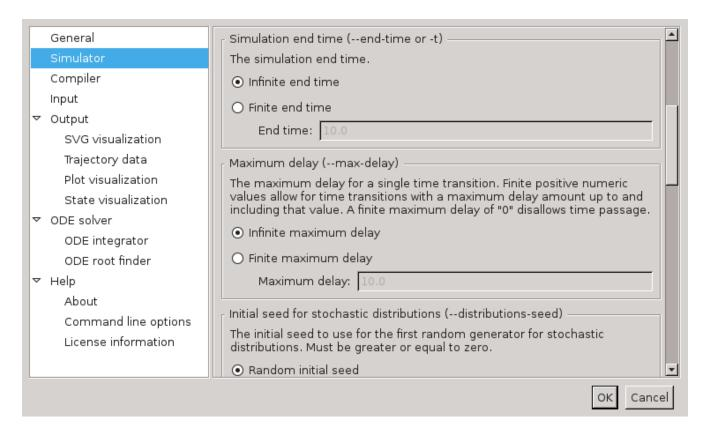
There, it is listed as *Simulator end time* option. After that name, the command line names of the option (--end-time and -t) are also listed. This makes it easier to link options in the option dialog with command line options.
