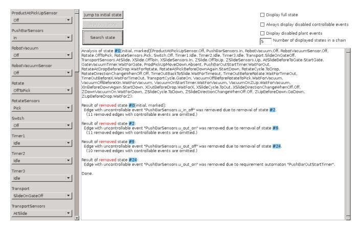
This is an example from a bigger system, where the supervisor is empty. The analysis of the initial state reveals that it was removed due to a removal of a chain of other states. State #24 was removed due to a requirement (reading from bottom to top), which caused the chain of states #9, #2, and eventually #0 to be removed.
