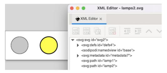
The visualization shows the two lamps. The first lamp is off, and has a silver background color. The second lamp is on and has a yellow background color. The lamp that is off has a thin border and the lamp that is on has a thicker border. The CIF specification also contains four CIF/SVG output mappings, two for the background colors of the circles and two for the thickness of the borders (strokes) of the circles.
