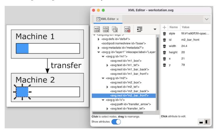
In the image, two machines are clearly visible. Each machine has a bar that shows the progress of the machine. Looking at the *XML Editor* window, we can see the bar has a background (box), and a foreground (front) rectangle. The width and fill color of the latter will be updated to reflect the machine's status.
