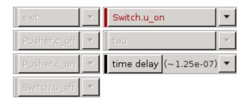
The events of the system are vertically listed, in alphabetical order, with event tau at the end, just before the [time delay], [reset], and [undo]. If there are too many elements to fit vertically, more columns are used. If things still don't fit, a horizontal scroll bar is shown.
