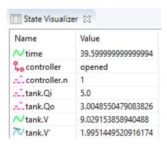
Unlike the SVG visualizer, which requires that the user makes an image of the system and couples the image to the specification, the state visualizer can be used directly, without any additional effort. All that is required to use it, is to enable it. The state visualizer is disabled by default, and can be enabled using the *State visualization* option (*Output: State visualization* category).
