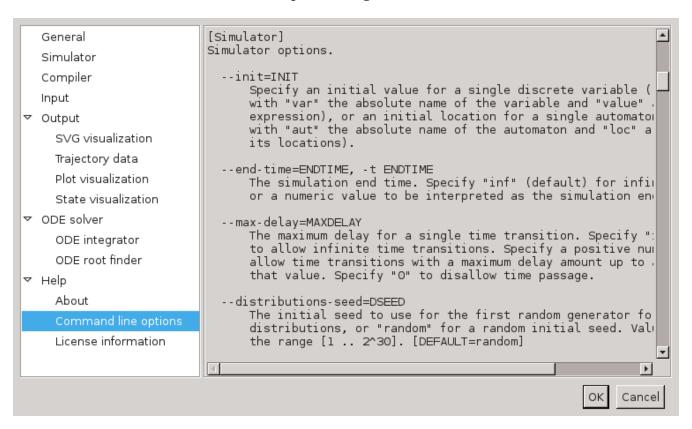
The option dialog shows the same help text as the command line --help and -h options. In this screenshot, you can see the help text of the --end-time or -t option. This particular option can also be configured using the option dialog. It is part of the *Simulator* category:
