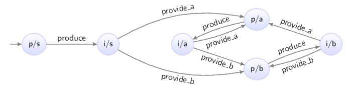
Now, whenever the provide\_a event is possible, the provide\_b event is also possible, and vice versa, just as in the producer automaton. The detect\_changeover automaton no longer restricts the occurrence of the events; it only monitors them.
