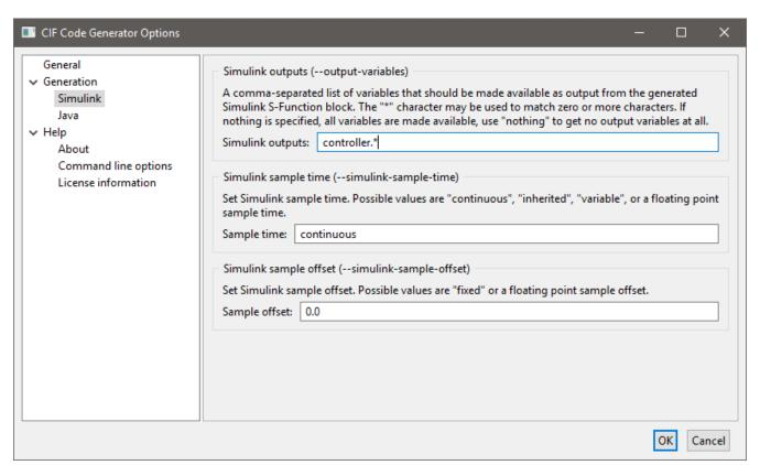
After clicking [OK], the CIF model is translated to C code. Code generation from the tank\_ctrl.cif files results in two output files. The tank\_ctrl.c file contains the generated C source code. The tank ctrl report.txt is a text file describing the data of the generated SFunction code:
