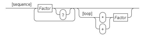
Note that together with | above and the empty sequence () below, you can write all loops using the + infix operator. The Examples section explains this as well.
