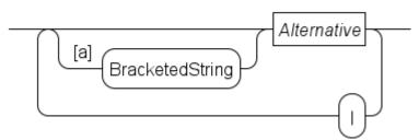
The BracketedString like [a] can be used to denote specific points in the diagram allowing you to refer to such points from the explanatory text.
