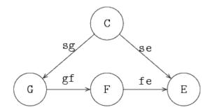
F is the factory being studied, generator 6 sends products into the factory, and exit process E retrieves finished products. The factory is tightly controlled by controller C that sends a signal to 6 or E before a product may be moved. The model is as follows:
