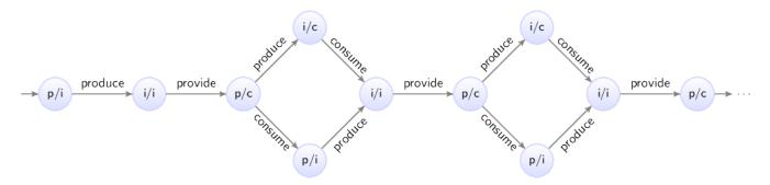
Here the circles represent the states of the specification, which are a combination of the states of the two automata. The labels of the circles indicate the state, as a combination of the first letters of the locations of the automata. The initial state is labeled p/i, as initially automaton producer is in its producing (p) location, and the consumer is in its idle (i) location. The arrows indicate the transitions,
