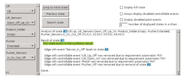
State **#7** has one outgoing edge, leading to state **#9** using event Sensor\_In\_Off. The last line with the removed controllable events displays a removed edge because destination state **#8** was removed.
