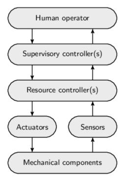
At the bottom are the mechanical components, such as motors, switches, levers and valves. Their operation can be steered through actuators and their state of operation can be observed through sensors. Resource controllers provide a first level of control. They may for instance correct for sensor jitter, translate continuous signals to discrete ones, or detect and even correct anomalous situations.
