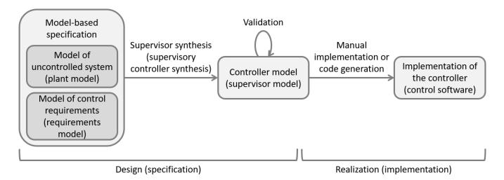
As with general model-based engineering, at the center is a controller model with a mathematical foundation. From the controller model, the control software can still be manually implemented or automatically generated.
