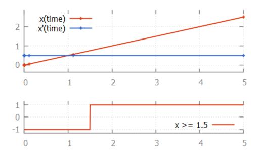
we see that at time 1.1111, the value of the guard is -1 (false). At time 5.0 it is +1 (true). That is, the guard changed value between two time points calculated by the integrator. If this is the case, the ODE solver tries to calculate the exact time point at which the guard changes its value. That is, it calculates the exact time point at which the guard function crosses the time axis, and thus has a root.
