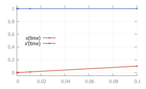
Here, the numerical integrator start with the initial value of continuous variable x, which is 0.0. For the initial value of variable time, which is also 0.0, it computes x', which is 1.0. It then slightly increases the value of variable time to say 1e-6. Assuming a linear continuous variable x, the value of variable x at that time is 1e-6 as well.
