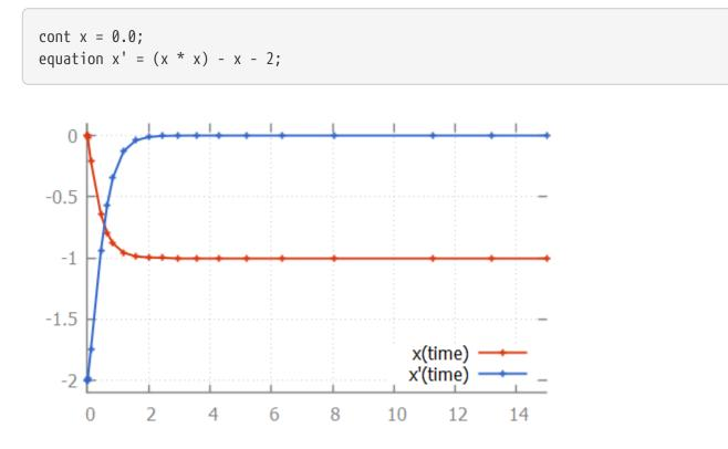
Here, we see how the step size is increased initially, as the linear approximation is good enough. As soon as we get to the bend, the step size is reduced to better approximate the actual values. After the bend, the step size is slowly increased again. The integrator internally uses a polynomial of a higher degree to approximate this differential equation.
