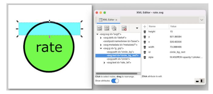
The SVG image visualizes a machine as a circle. The rate of the machine is visualized as the background of the circle. The higher the rate, the more the circle is filled.
