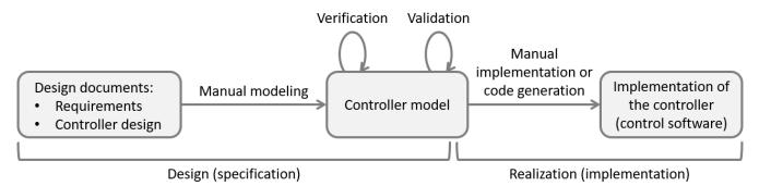
The verification-based engineering process is very much similar to the model-based engineering process. The only difference is the way the verification of the controller (model) against its specified requirements is performed. Verification-based engineering uses formal verification, or model checking, to mathematically prove a certain property holds. Such properties could for instance be the absence of deadlock or livelock, or that a bridge may only open if its corresponding traffic lights
