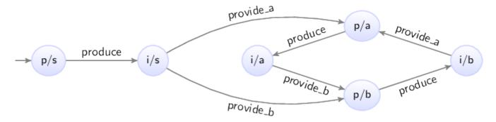
The states are labeled with the first letters of the names of the current locations of the automata. Note how the i/a and i/b locations only have outgoing transitions for either the provide\_a transition or the provide\_b transition.
