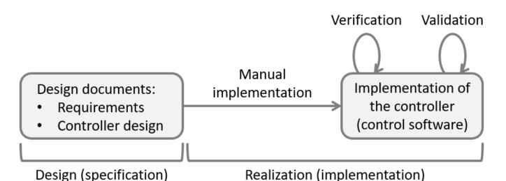
Traditionally, controllers are first specified in design documents. They for instance list their functional and safety requirements, describe their control states and indicate when the controller should actuate the various actuators depending on changing sensor signals.
