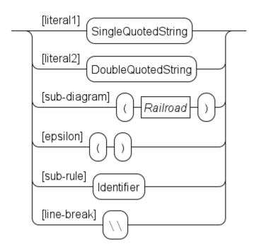
The [literal1] and [literal2] choices show the text of the string. Surrounding quotes are dropped. There are two forms of literals to simplify using single or double quote literals in the diagrams. The [sub-diagram] choice allows nesting of sequence, choice, and repetition, enabling construction of more complicated diagrams. The [epsilon] choice is the empty sequence. The [sub-rule] choice enables giving the name of another diagram to process.
