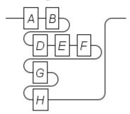
The double backslash breaks the 'line' and it continues below on the next line. You cannot break the empty sequence, and each row must have at least one node.
