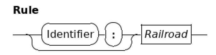
Obviously something is not right here as various lines and arcs are not connected properly to each other. Unfortunately, what the cause for these misalignments is doesn't become clear. For example, the arc at the left is clearly above the line it should connect to, but is the arc too high or the line too low? To decide where the cause of the problem lies, you need to do some analysis first.
