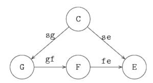
F is the factory being studied, generator G sends products into the factory, and exit process E retrieves finished products. The factory is tightly controlled by controller C that sends a signal to G or E before a product may be moved. The model is as follows:
