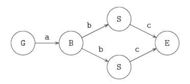
Generator process **G** sends items via **a** to buffer process **B**, and process **B** sends the items in a first-in first-out manner to the servers **S**. Both servers send the processed items to the exit process **E** via channel **c**. The inter-arrival time and the two process times are assumed to be stochastic, and exponentially distributed. Items can pass each other, due to differences in processing time between the two servers.
