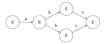
Generator process 6 sends items via a to buffer process B, and process B sends the items in a first-in first-out manner to the servers S. Both servers send the processed items to the exit process E via channel c. The inter-arrival time and the two process times are assumed to be stochastic, and exponentially distributed. Items can pass each other, due to differences in processing time between the two servers.
