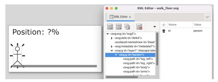
The text label is to be used to show the position of the person, as a percentage. The left position is represented as 0%, and the right position is represented as 100%. The id of the text label is pos\_txt.
