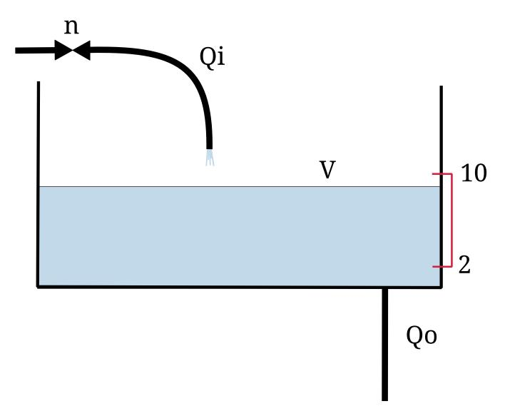
The water in the tank has volume V. At the bottom of the tank is a pipe where water flows away with speed Qo. At the top is a pipe with valve n that can be open or closed. The Qi variable denotes the speed of water flowing into the tank. The equations that hold in this system are:
