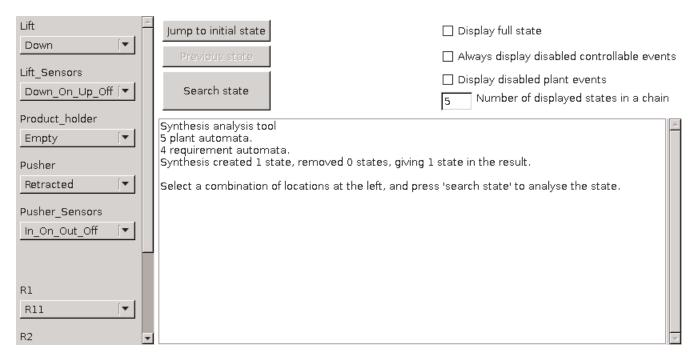
At the left, all automata with their initial location are shown. You can select a different supervisor state by changing these locations. At the top, in the middle, there are three buttons. The bottom [Search state] button is used to search the information about a supervisor state selected at the left. The [Jump to initial state] button resets the automata to their initial state, useful when you want to start again. The middle [Previous state] button is disabled now, but allows you to go back
