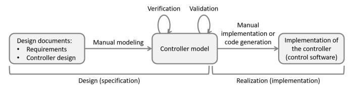
At the center is a controller model, a model of a controller that unambiguously specifies how the controller works. It precisely specifies how the state of the controller changes when a sensor signal changes, and under what conditions and in which states an actuator may be turned on or off. Ideally, the model has a mathematical foundation. It may for instance be modeled as one or more state machines.
