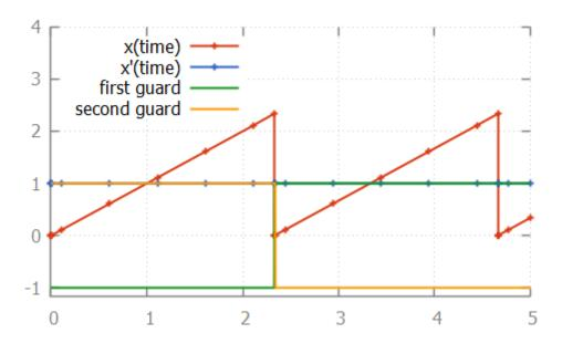
The difference with the original specification is the guard of the edge. In the original specification, the and binary operator is used, making it a single guard. In the new specification, a comma (,) is used, which constructs two separate guards. Both guards can be individually checked by the root finding algorithm. As shown in the image, each of the guards changes value only once.
