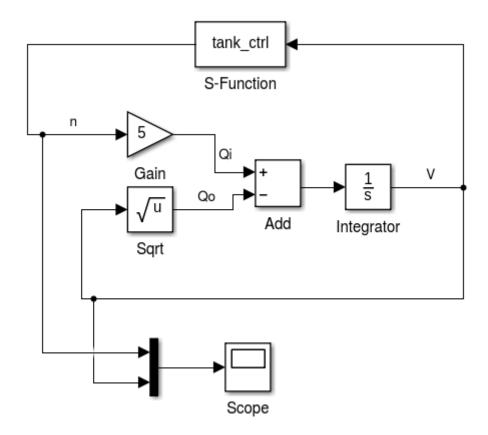
In the middle the equations are modeled. The output of the equations is V, which is fed into the S-Function block with the CIF controller at the top. The controller computes n which is an input for the equations.
