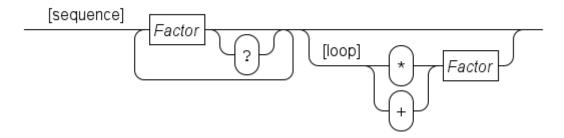
Note that together with | above and the empty sequence () below, you can write all loops using the + infix operator. The Examples section explains this as well.
