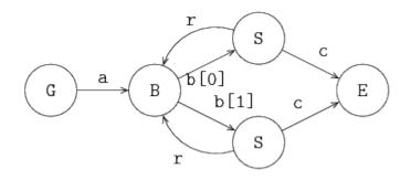
In this model, the servers 'pull' an item through the line. The model is:
