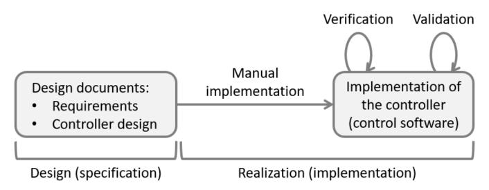
Traditionally, controllers are first specified in design documents. They for instance list their functional and safety requirements, describe their control states and indicate when the controller should actuate the various actuators depending on changing sensor signals.
