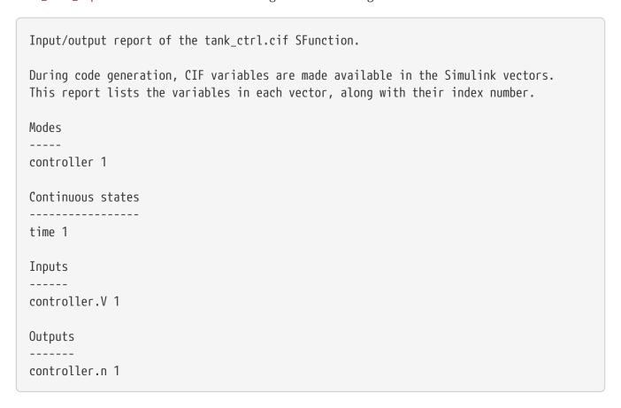
The report shows which CIF variables are available at each vector. The *Inputs* and *Outputs* are the most interesting. Here it shows that V is the only input variable, n is the only output variable, and they are both the first value in their vector. This is what you would expect for such a small system.
