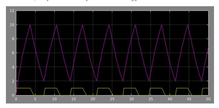
The volume fluctuates between 2 and 10, at the bottom is the control signal n.
