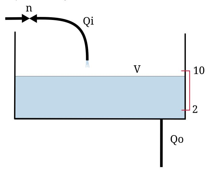
The water in the tank has volume V. At the bottom of the tank is a pipe where water flows away with speed Qo. At the top is a pipe with valve n that can be open or closed. The Qi variable denotes
