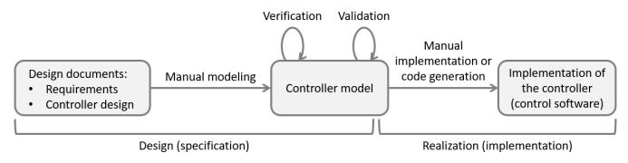
The verification-based engineering process is very much similar to the model-based engineering process. The only difference is the way the verification of the controller (model) against its specified requirements is performed. Verification-based engineering uses formal verification, or model checking, to mathematically prove a certain property holds. Such properties could for instance be the absence of deadlock or livelock, or that a bridge may only open if its corresponding traffic lights
