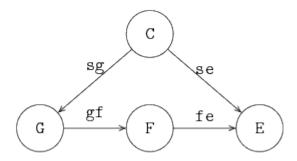
F is the factory being studied, generator 6 sends products into the factory, and exit process E retrieves finished products. The factory is tightly controlled by controller C that sends a signal to 6 or E before a product may be moved. The model is as follows:
