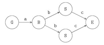
Generator process G sends items via a to buffer process G, and process G sends the items in a first-in first-out manner to the servers G. Both servers send the processed items to the exit process G via channel G. The inter-arrival time and the two process times are assumed to be stochastic, and
