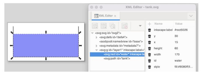
The image features a tank (black lines) and the water in the tank (blue rectangle). The water rectangle is selected. In the *XML Editor* window, you see the position as SVG represents it. It shows 15 for the x position and 30 for the y position. These values are relative to the upper left corner of the canvas.
