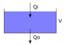
Variable V models the water volume of a tank. The water volume of the tank changes based on the incoming flow of water Qi and outgoing flow of water Qo. The tank can be modeled using the following CIF specification:
