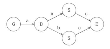
Generator process G sends items via a to buffer process B, and process B sends the items in a first-in first-out manner to the servers S. Both servers send the processed items to the exit process E via channel c. The inter-arrival time and the two process times are assumed to be stochastic, and
