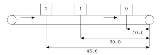
Three items are placed on the conveyor. For simplicity, assume the conveyor is 60.0 meter long and has a speed of 1 meter per second. An item thus stays on the conveyor for 60.0 seconds.
