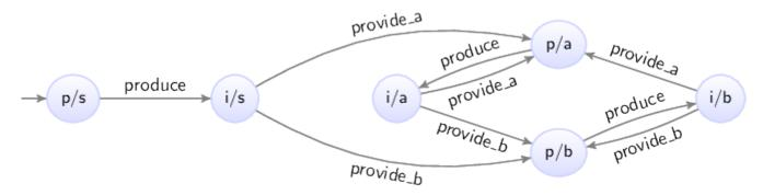
Now, whenever the provide\_a event is possible, the provide\_b event is also possible, and vice versa, just as in the producer automaton. The detect\_changeover automaton no longer restricts the occurrence of the events; it only monitors them.
