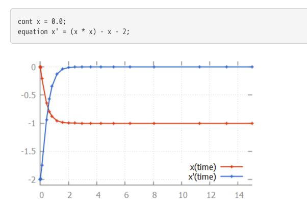
Here, we see how the step size is increased initially, as the linear approximation is good enough. As soon as we get to the bend, the step size is reduced to better approximate the actual values. After the bend, the step size is slowly increased again. The integrator internally uses a polynomial of a higher degree to approximate this differential equation.
