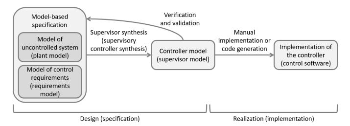
As with general model-based engineering, at the center is a controller model with a mathematical foundation. From the controller model, the control software can still be manually implemented or automatically generated.
