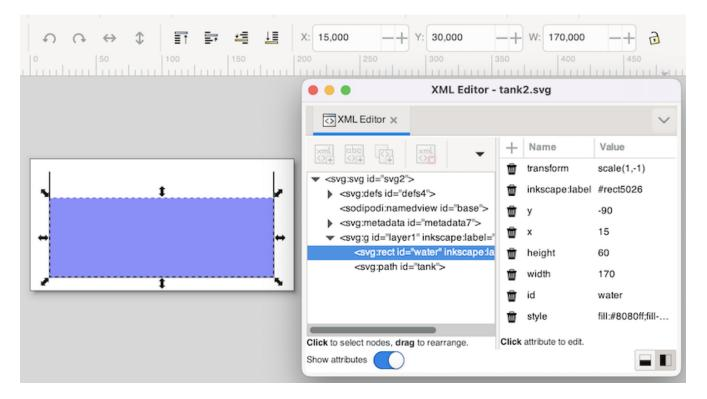
This SVG image is the same as the original SVG image for this example, but with an inverted y-axis,
