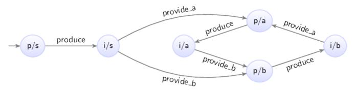
The states are labeled with the first letters of the names of the current locations of the automata. Note how the i/a and i/b locations only have outgoing transitions for either the provide\_a transition or the provide\_b transition.
