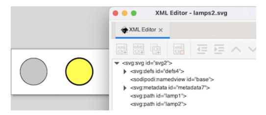
The visualization shows the two lamps. The first lamp is off, and has a silver background color. The second lamp is on and has a yellow background color. The lamp that is off has a thin border and the lamp that is on has a thicker border. The CIF specification also contains four CIF/SVG output mappings, two for the background colors of the circles and two for the thickness of the borders (strokes) of the circles.
