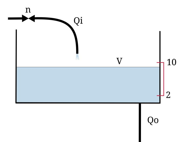
The water in the tank has volume V. At the bottom of the tank is a pipe where water flows away with speed Qo. At the top is a pipe with valve n that can be open or closed. The Qi variable denotes the speed of water flowing into the tank. The equations that hold in this system are:
