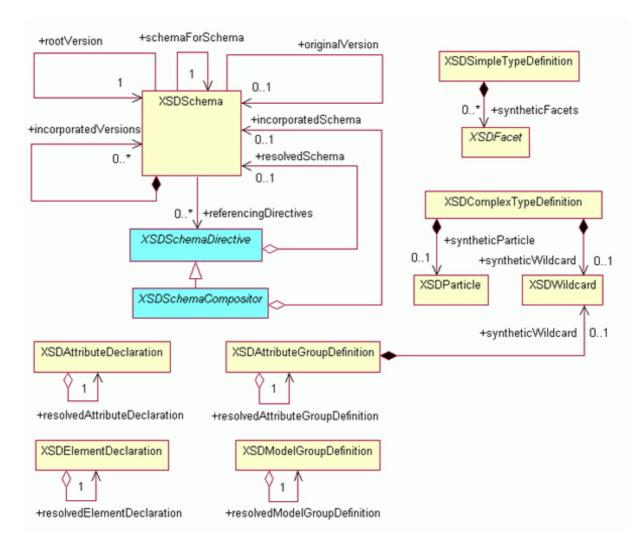
The figure above illustrates how some concrete components resolve to the other concrete components:
