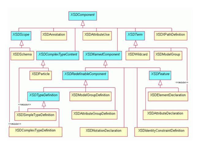
The figure above displays the hierarchy of the XML Schema Infoset model. The classes in light blue represent abstract classes, whereas the classes in light orange represent the concrete classes. Here is a short description of some of the classes that you will need to understand:
