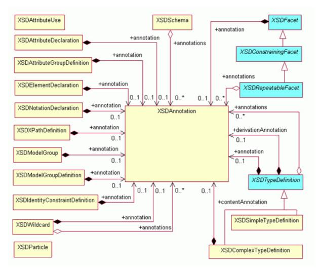
The figure above illustrates how the XML Schema components are annotated, which correspond to xml schema <xsd:annotation ...> tag.
