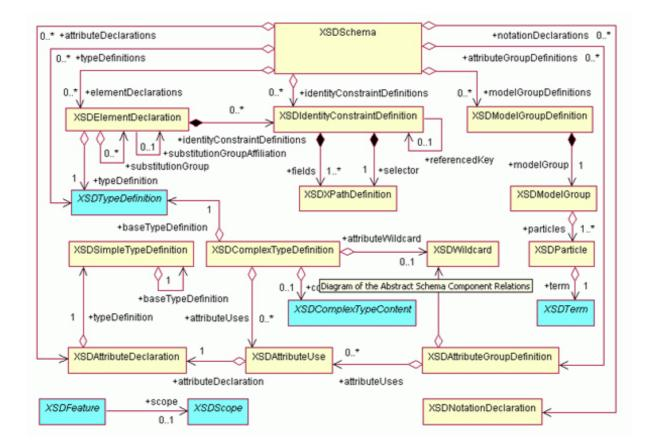
The figure above is very similar to the standard *non-normative Schema Components Diagram.* This diagram is very complex, so the main thing to notice are the white diamond relationships, which are the shared pseudo-containment relationships and are computed from other relations within the model.
