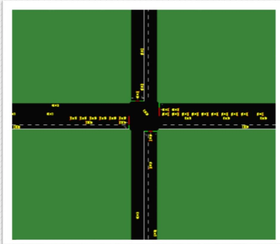
The single intersection scenario used in the MOYCOT project to obtain parameters needed for MPC traffic lights controller.
